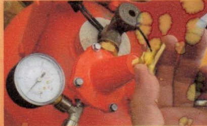
Turn pressure gauge to approximately 1-3 PSI for lighting
