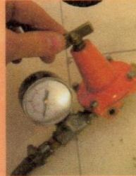
Unscrew the regulator out as far as possible (anti-clockwise)
