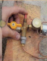
Ignite lighting device and hold near burner tip. Press flame failure starter button to let gas through
