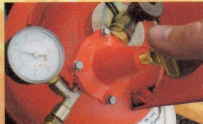
Gas pressure can be adjusted to suit your firing 2 - 10 PSI is about normal.
