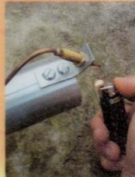
Ignite lighting device and hold near burner tip. Press flame failure starter button to let gas through
